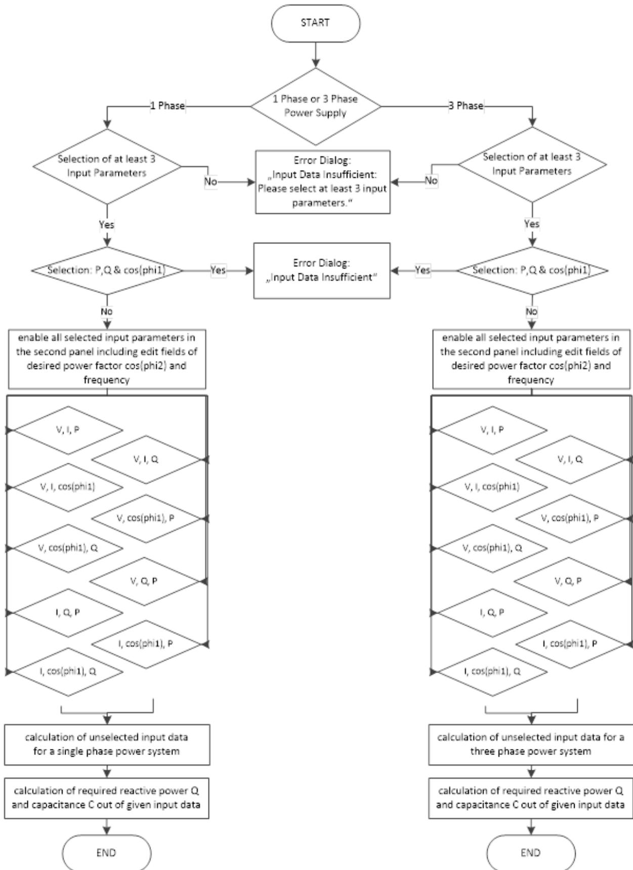
Figure 1: Flowchart Representing the Calculations Done in GUI
