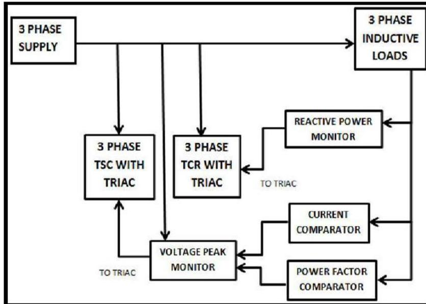
**Figure 6: Block Diagram of SVC with Feedback**
