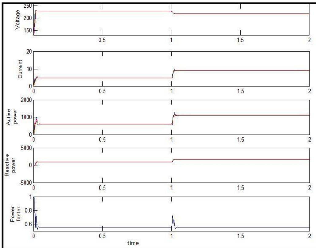
**Figure 3: From Top to Bottom - Voltage, Load Current, Active Power, Reactive Power, Power Factor of Phase a**
