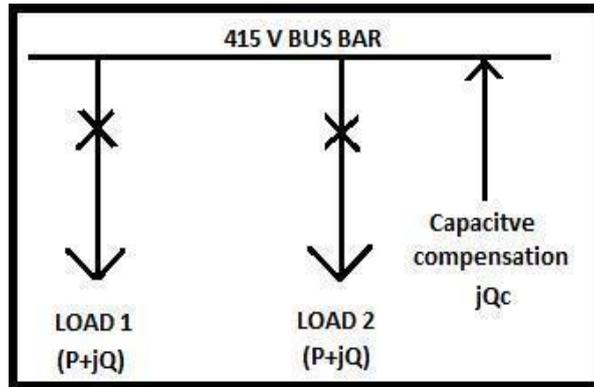
**Figure 2: Single Line Diagram of Laboratory under Study**
